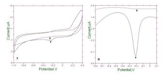
Figure 1. (A) CVs of GSH and (B) DPVs of GSH in PBS (pH 7.4) at (a) SWCNT/GCE modified sensor and (B) bare GCE vs. Ag/AgCI.
